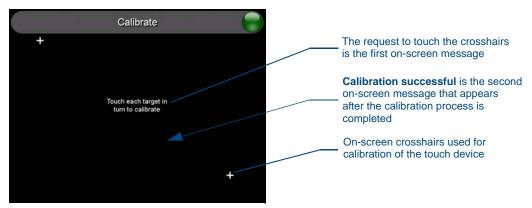
FIG. 89 Touch Panel Calibration Screens
